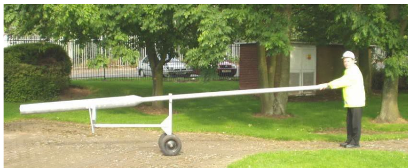
Figure 10-2 - Carrier and column ready for moving
